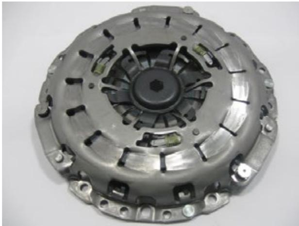
The locking plate can only be removed from the cover assembly after fitment by engaging an Allen-head socket wrench or key into the centre hole of the locking plate, and rotating the locking plate in order to disengage it from the cover assembly. A slight click may be heard from the cover assembly when the locking plate is removed.
