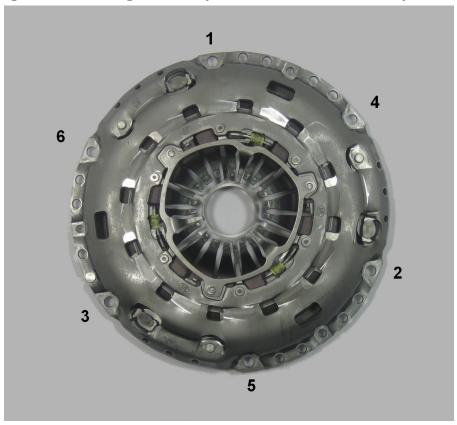
Always ensure the cover is located on the dowel pins (if applicable) prior to tensioning the pressure plate bolts.
