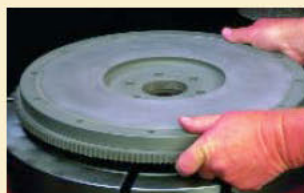
2. Lay the flywheel on the adapter
