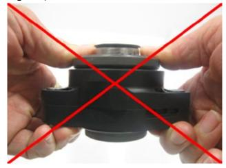
In some applications compressing the cylinder can dislodge the rear seal of the cylinder (see picture below)
