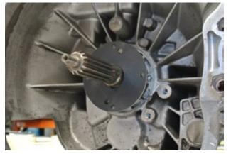
Mount the alloy adapter plate on top of the shim or straight to the transmission using the four M6 bolts supplied. Ensure the locating collar is facing outwards. The threaded holes for mounting the release bearing must be toward the top and bottom.
