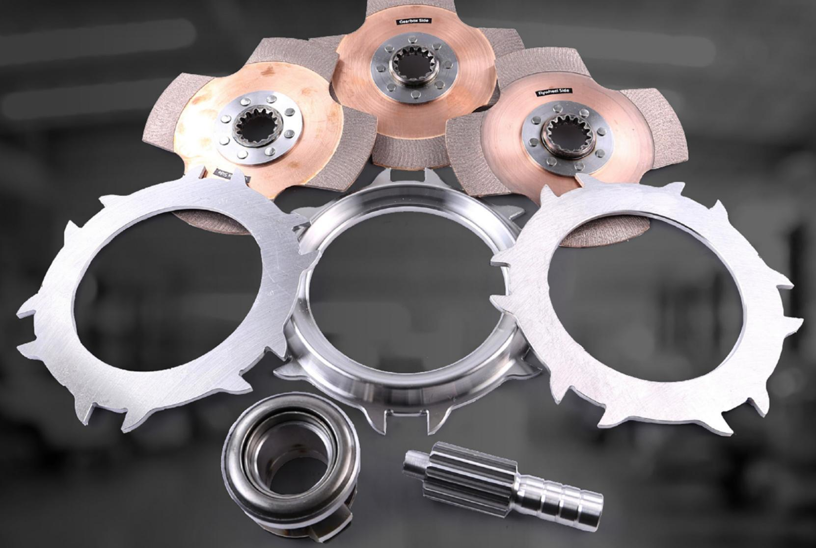
Xtreme Clutch multi-plate kits are designed and engineered for high performance street and motorsport applications where a high torque capacity is critical. These multi-plate upgrades are available in a range of configurations including organic, ceramic and carbon friction materials and with various disc quantities.
