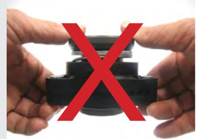
Do not depress a CSC by hand prior to fitting – NEVER compress a CSC by hand to replicate the bearing movement this can damage the internal seals, as the cylinder has no hydraulic fluid within the system.
