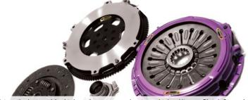
Primarily designed for high performance road-going vehicles, Xtreme Clutch Stage 1 clutch kits deliver substantial increases in performance and power holding capabilities whilst retaining ease of drivability. These kits include an organic friction disc with rigid or sprung options available.
