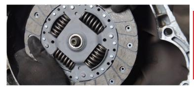
Replacing a clutch friction plate or a thrust bearing in isolation & not as part of a matched kit can potentially cause clutch operation failure.
